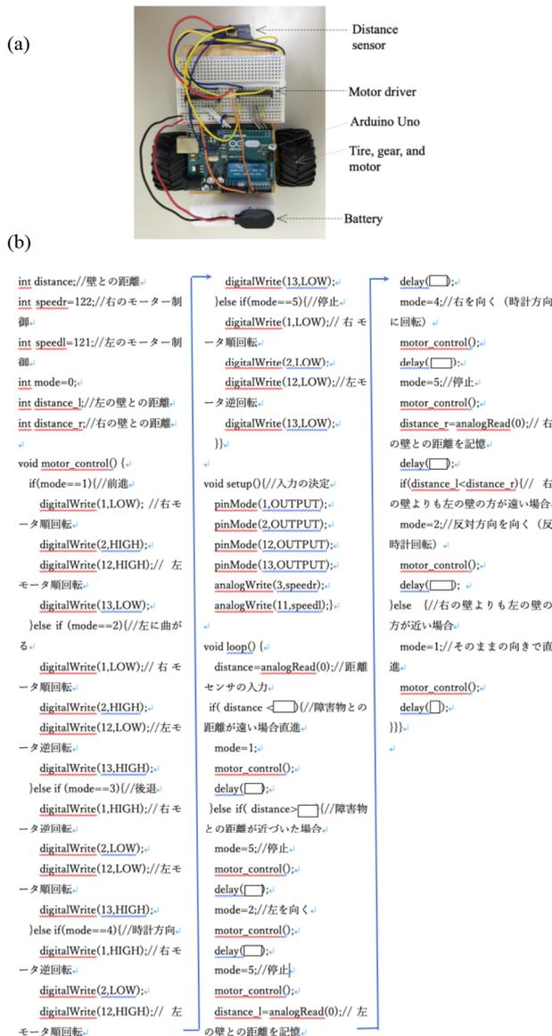
Figure 1 Examples of an autonomic robot car capable of getting out of labyrinth (a) and a control program installed in Arduino UNO (b) developed by student.
